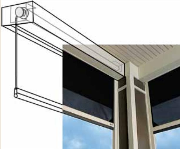
*Recessed mount showing detail of cavity contents*
